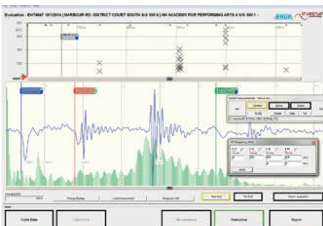
➤ Partial discharge measurement unfiltered
